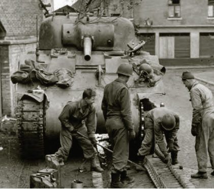
Installing track extensions on an M4, called grousers or duckbills
