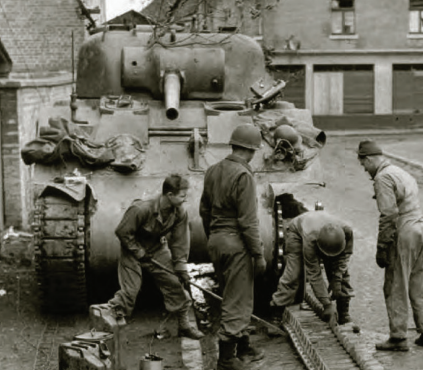
Installing track extensions on an M4, called grousers or duckbills
